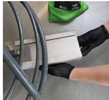
3. Slide Quick Change blade to the standard 6" finishing blade
