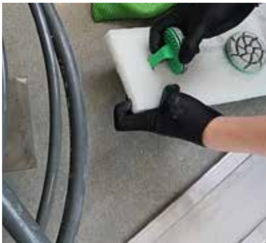
1. Attach diamond discs to the mounting pad through the pre-cut slits
